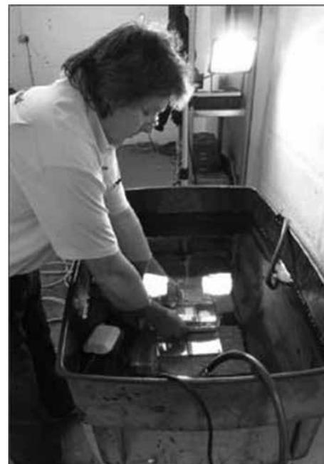
**Fig 4:** Measuring ambient light prior to MPI
