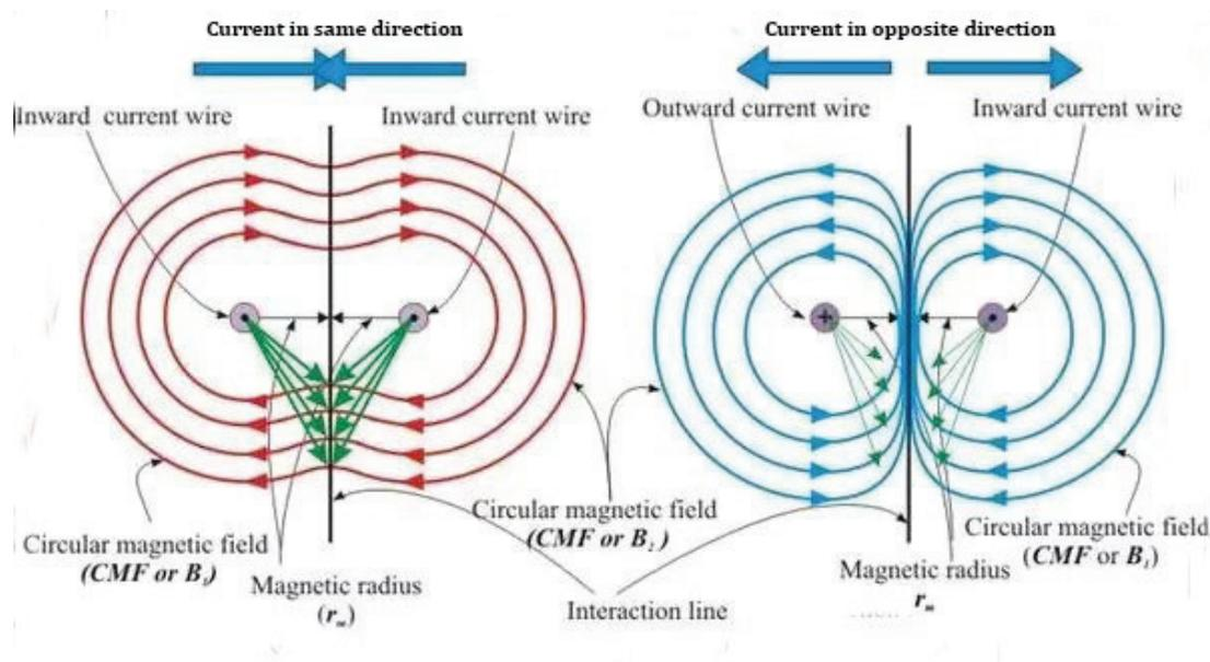
**FIG 16: Forces between two wires containing opposing current showing flux compression.**
