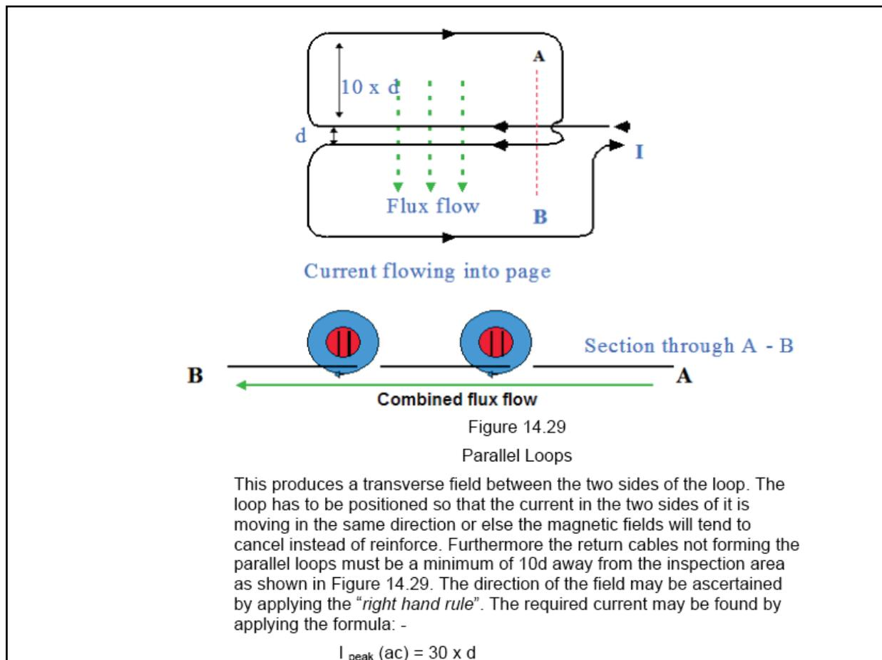
**FIG 5: Parallel Loops as described in TWI Subsea Inspection Manual April 2006.**
