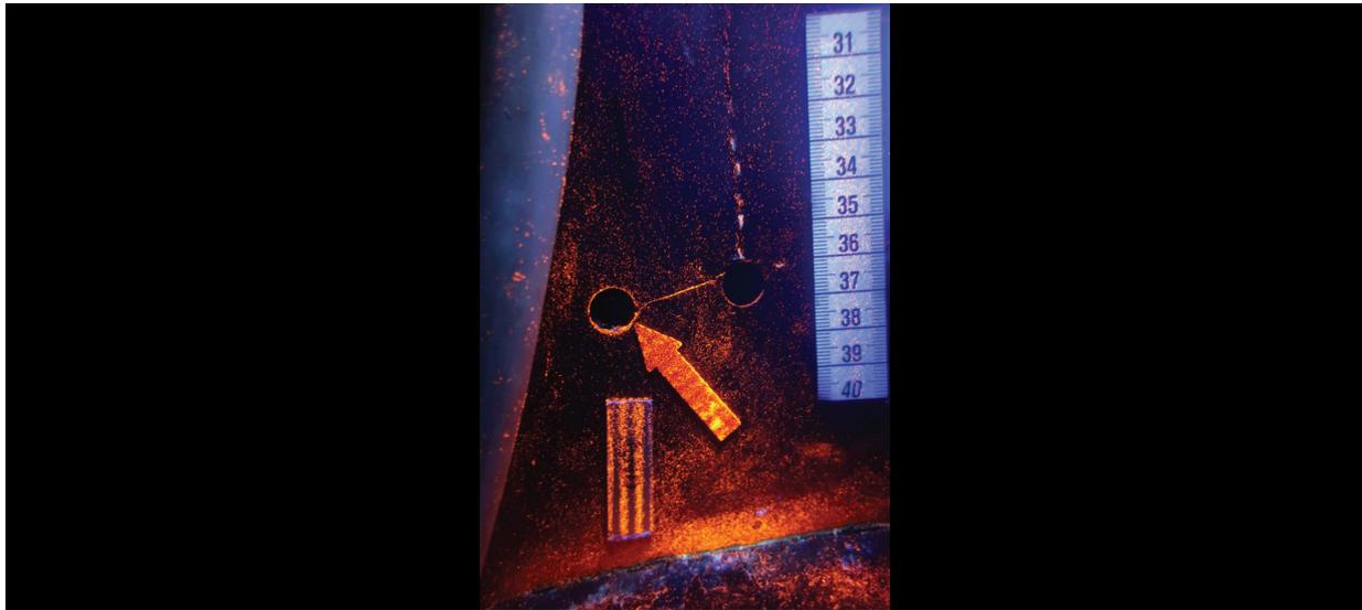
**FIG 14:** Close up showing vertical crack and horizontal transverse branch: UV-A light.
