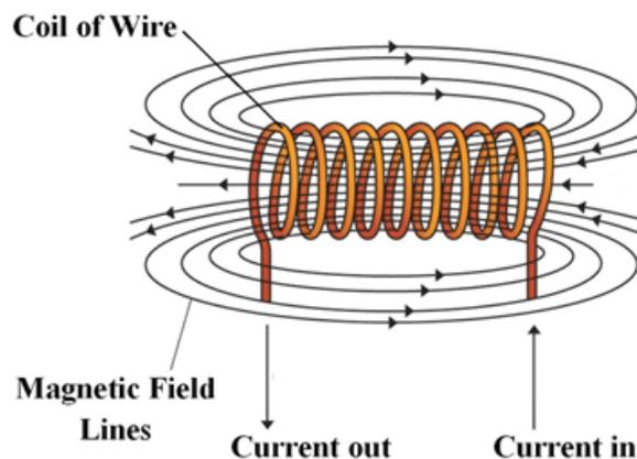
**FIG 4: Magnetic field created by an electrical current running through a coil of copper wire.**
