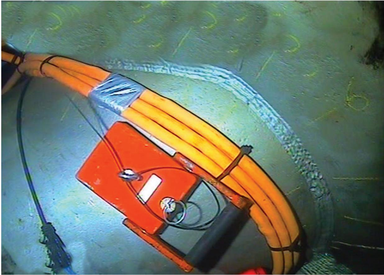
**FIG 10: Compressed Flexible Cable Bundle deployed over horizontal structural member.**
