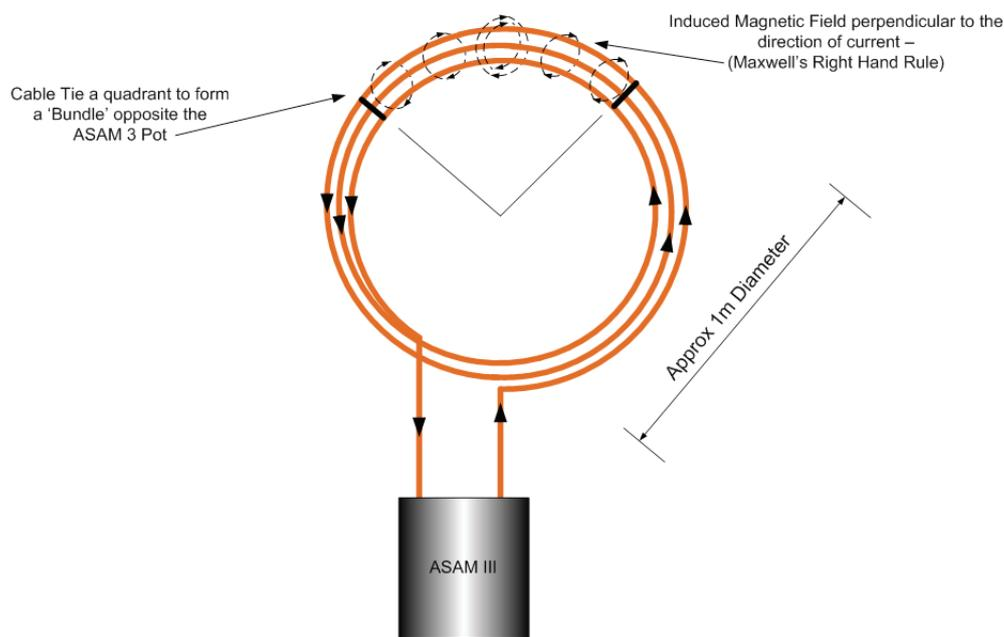
**FIG 6: The Quadrant System of A.C. Flexible Coil DESIGN.**
