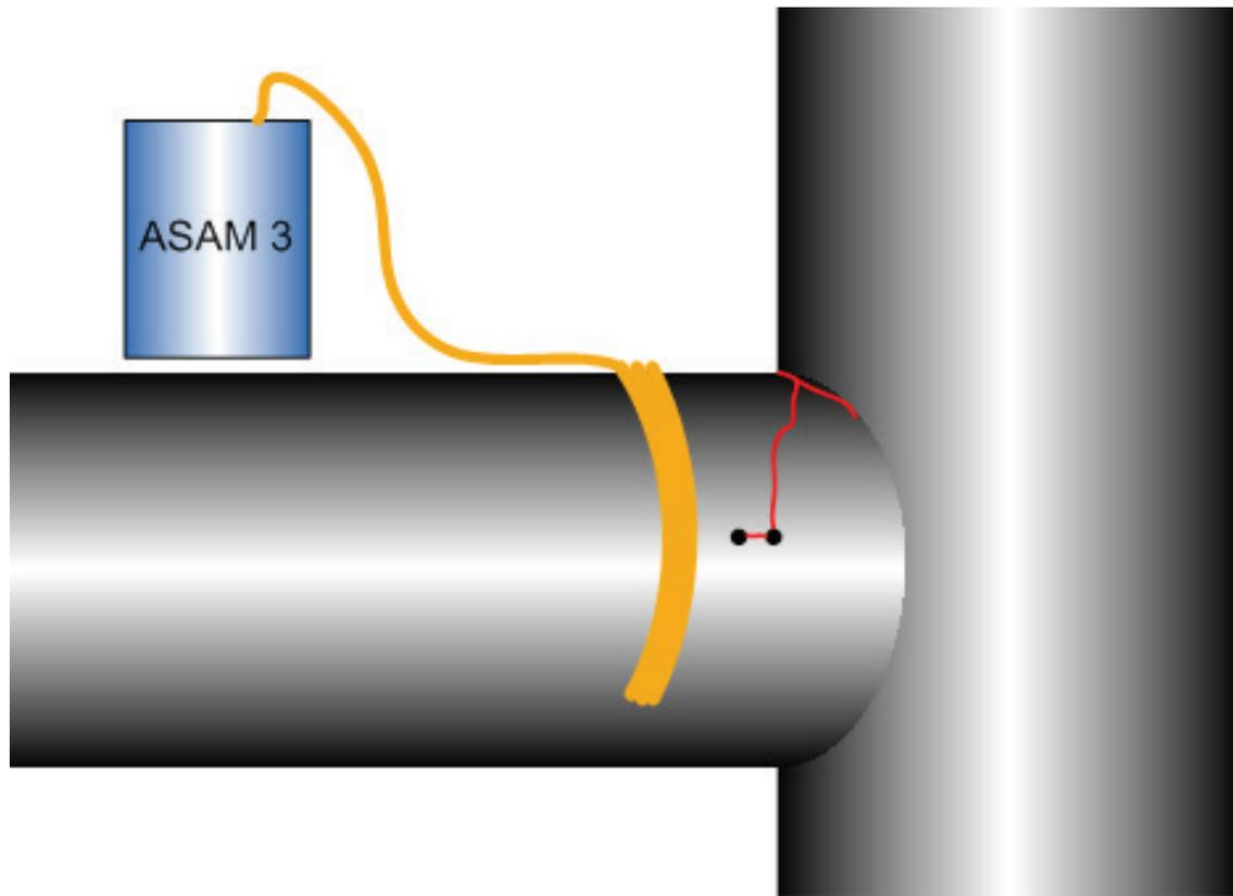
**FIG 11: Discontinuities revealed at angles approaching 90 degrees.**
