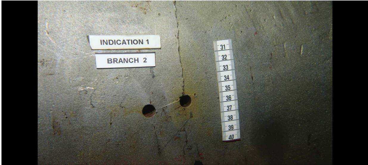
**FIG 13:** Close up showing vertical crack and horizontal transverse branch: ambient light.
