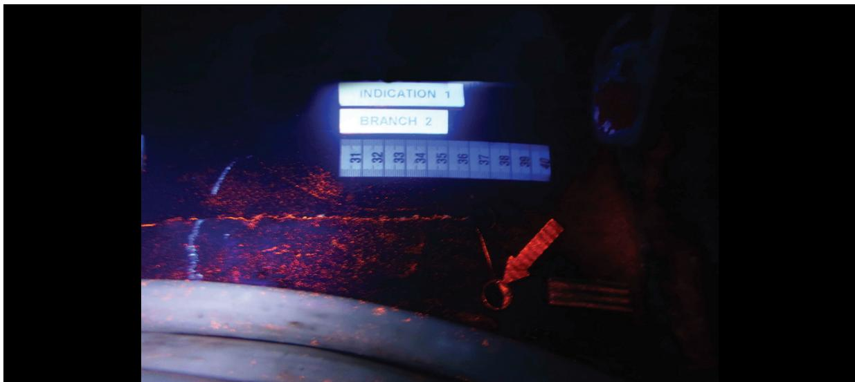
**FIG 15:** Detail of indication at 90 degrees with view of cable in lower screen.
