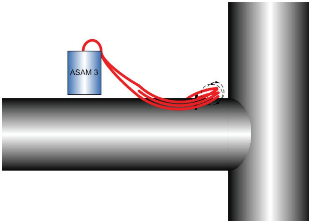
**FIG 7: The Quadrant System of A.C. Flexible Coil deployment.**
