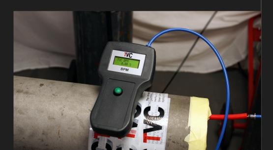
designed for quick spot checks when purging
