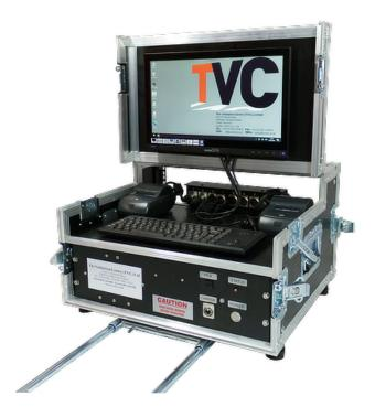
The ALX III Series weld monitoring system can monitor voltage and current as standard. It can also be configured to monitor wire feed speed, gas flow, travel speed, type 'K' contact temperature, purge oxygen level, laser depth, multi-channel temperature, and wireless transducers and sensors connectivity.
