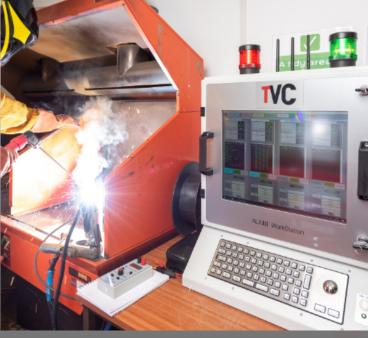
Wireless connectivity: transducers and sensors The ALX III digital wireless sensor network allows battery-powered, application-specific transducers to be connected to ALX III units. Currently, there are specialist wireless sensors and transducers available for temperature, wire feed speed, travel speed, angle and position, gas flow measurement, and weld height.
