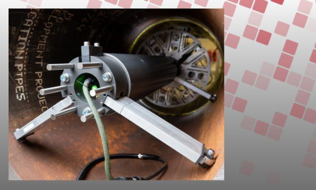
The CALSIS system can be deployed in three ways: attached to the rear of an ILUC, using a remote crawler vehicle, or manually using a push rod. Each system has both wireless and hard-wired connectivity options. When used wirelessly, a battery pack can also be supplied, which can power the CALSIS system and a remote crawler.
