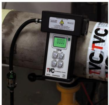
Additionally, a remote flow control box can be connected to the output of the HPM, which allows for automated purging of any inert welding gas. Control of purge gas flow ensures quick, accurate, and efficient purging, which can improve the quality of welds, reduce the risk of weld failures, and save money.
